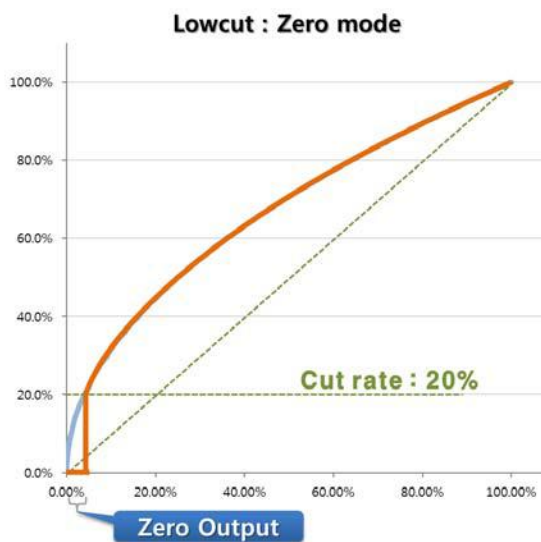
[Figure 6-13] Lowcut mode comparison
