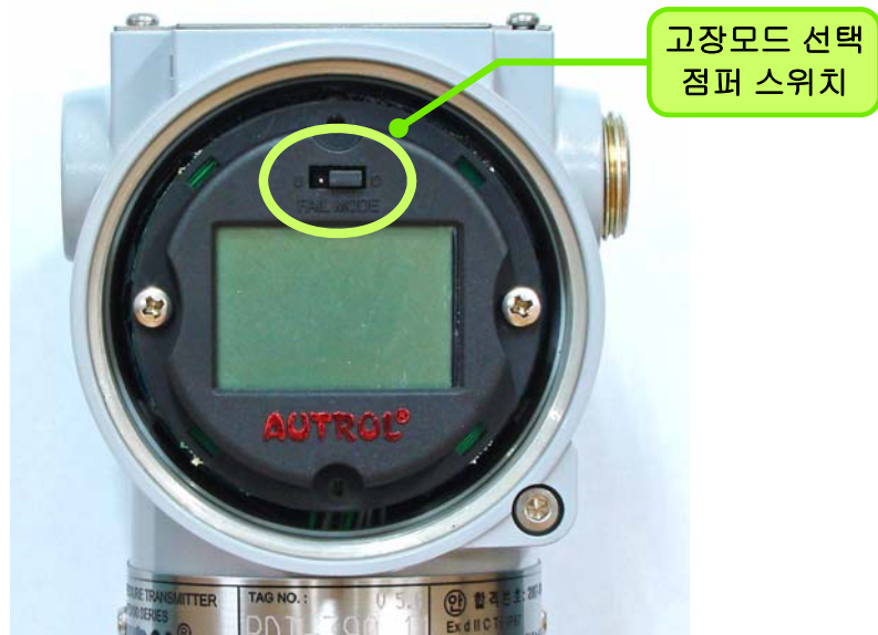
[Figure 6-7] Fail Mode Selection Jumper Switch in the CPU Module
