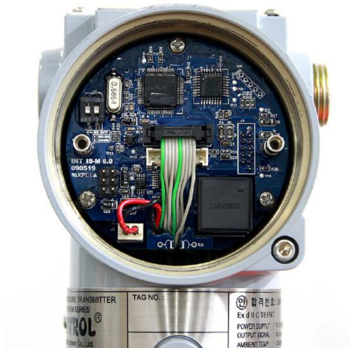
[Figure 7-1] Electronic circuit module
