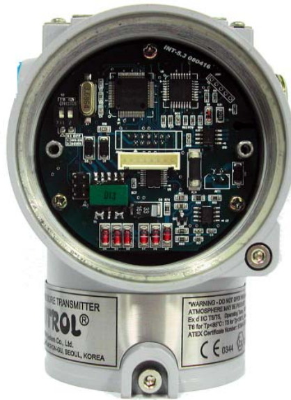
Figure 6-3 Structure of Electronics Module inner Transmitter
