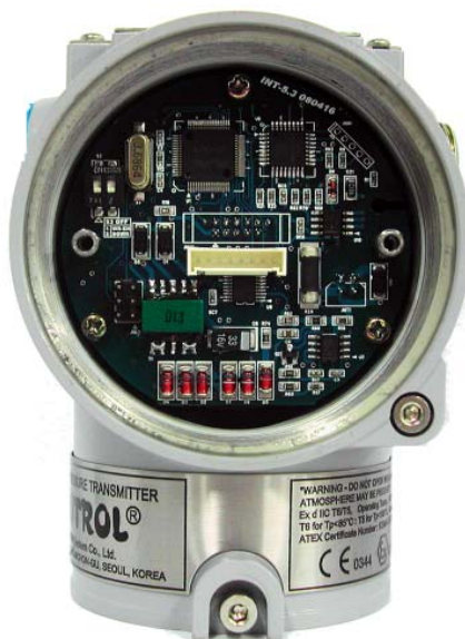
Figure 6-3 Structure of Electronics Module inner Transmitter
