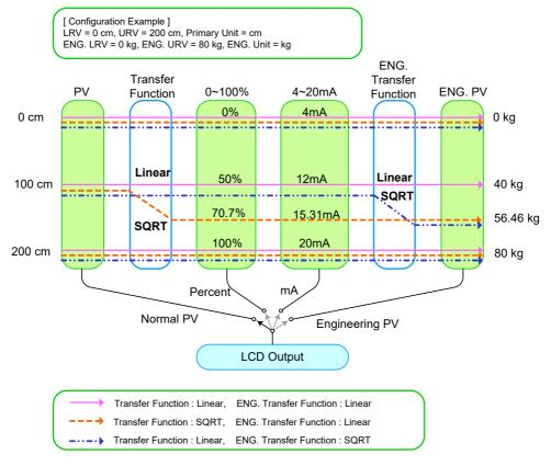
[Figure 1-1] Measured value processing procedure
