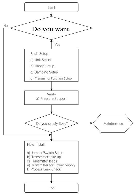
[Figure 4-1 Installation Flow Chart]
