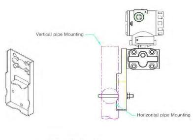
Horizontal Mounting Type 2" Pipe Mounting Bracket Model: Flat Type
