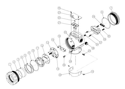
Figure 1-1. Model APT 3100 Transmitter Exposed View (Housing)
