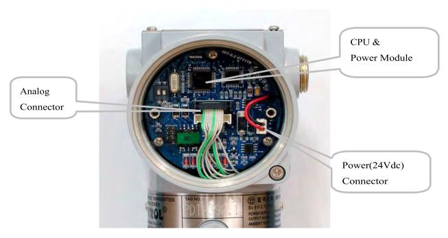
Figure 6.3 Structure of Electronics Module inner Transmitter
