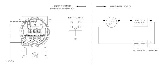
[Figure 4-3 Connection between Transmitter and Power Supply]
