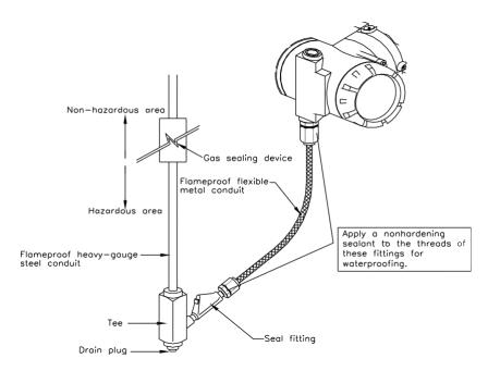
[Figure 4-4b Typical Wiring using Flameproof Packing Adapter]
