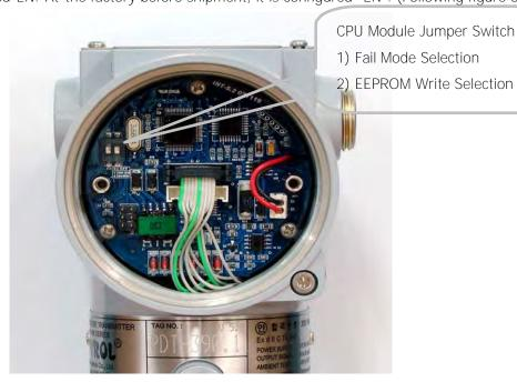
Figure 3-3. CPU Module Fail Mode, EEPROM-Write Selection Jumper Switch
