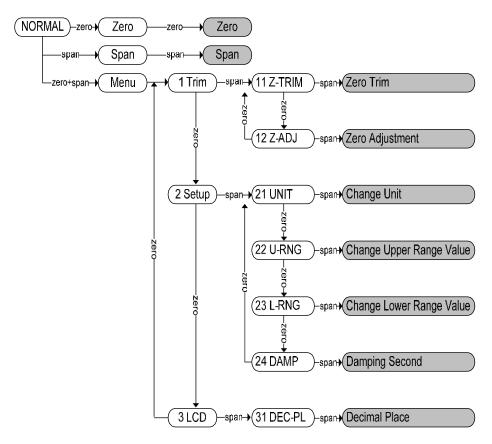
[Menu Tree of ZERO+SPAN Button Function]
