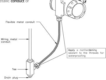
[Figure 4-4a Typical Wiring using Flexible Metal conduct]
