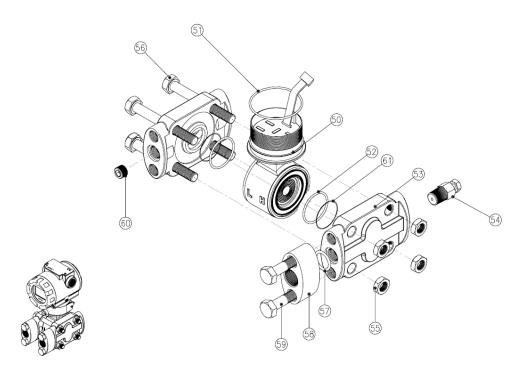
Figure 1-5. Model APT 3100 Exploded View (Sensor Module-H)
