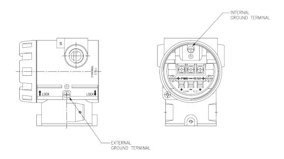
APT3100 SMART PERSSURE TRANSMITTER INTERNAL AND EXTERNAL GROUND TERMINAL
