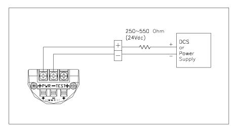
Figure 4-2 Connection with Terminal Board of Transmitter
