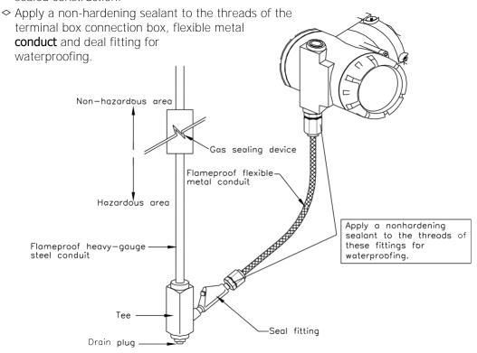
[Figure 4-4c Typical Wiring using Flameproof Metal **conduct**]
