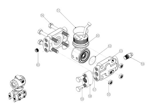
Figure 1-3. Model APT 3100 Exploded View (Sensor Module-D,G,L)
